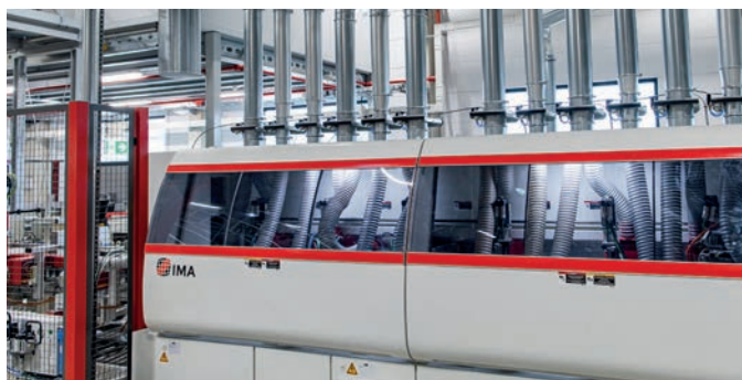
► Plant 2 Fully automated edge coating (glue or zero-joint edge)
