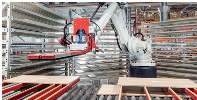
► Plant 2 Intermediate storage with robot-controlled sorting
